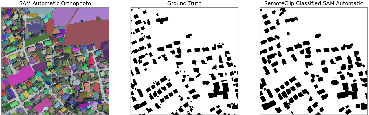
Figure 6. Example prediction on BBD of SAM Automatic classified with RemoteCLIP.
