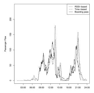
Figure 5: Results of RSSI and time-based Wi-Fi pedestrian flow estimations at a single day compared with boarding pass scans
