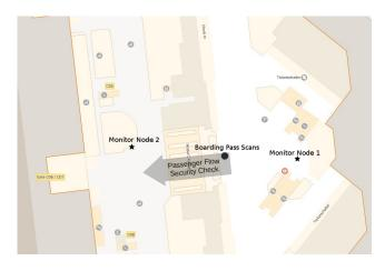
Figure 1: Map<sup>2</sup> of the testbed indicating the passenger flow through the security check, and the locations of monitor nodes, and boarding pass scans
